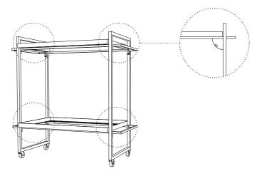
4. Aline the frame to create a right angle, than tighten all screws.
