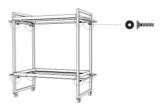
3. Screw in the bottom level screws, but don't tighten the screws completely.
