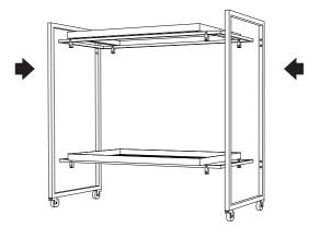
1. Place vertical frames in between the horizontal ones that all holes align.
