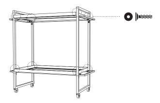
2. Screw in the top level screws first, but don't tighten the screws completely.
